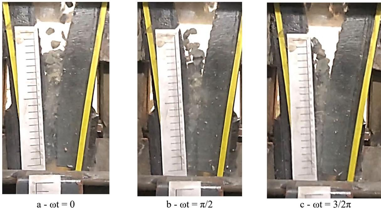
Figure 4 – Material movement in the grinding zone
