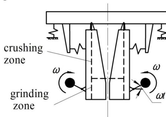
Figure 2 – Structural scheme of a vibratory jaw crusher
