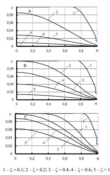
Figure 3 - Concentration of the component in the cross sections of the tube (k = 0.0001 m/s)
