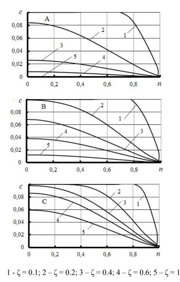
Figure 4 - Concentration of the component in the cross-sections of the tube (k = 0.001 m/s)
